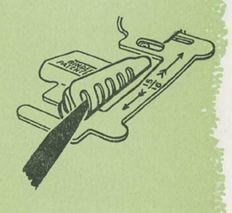
After the regular presser foot has been removed, replace it with the Attachment Foot. Then fasten the Binder to the foot. If you are using commercial single fold binding, cut the end to a long, thin point so that it can be drawn easily through the correct slot. Insert this pointed binding into the top outside slot. After inserting the point of the binding in the slot, use your stiletto to push the binding gently toward the needle.
