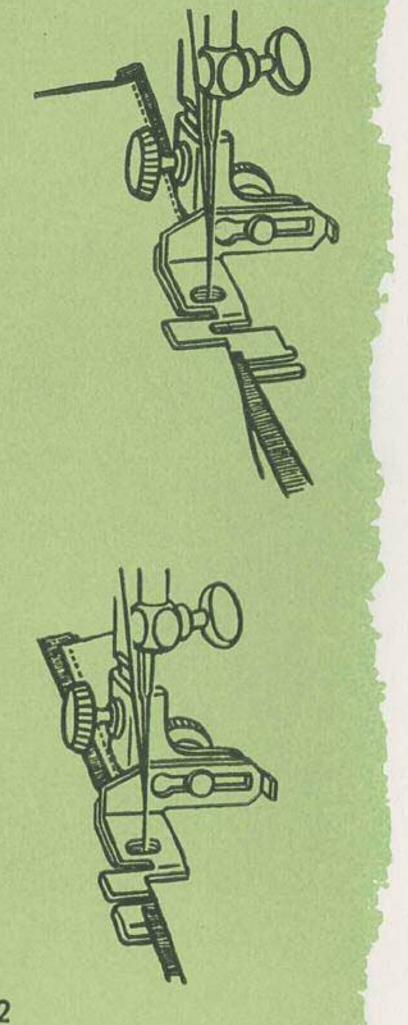
When using a piping to trim an article, the piping is put in slot 3. For a wide piping, the fabric is placed in slot 4 and the fold of the piping is to the left of slot 3. However, for a narrow piping, the fabric is placed in slot 2 and the folded edge of the piping is to the right in slot 3. Slot 5 is used as a guide when stitching a French seam.
