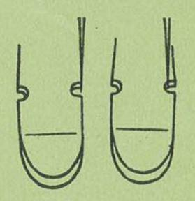
If you wish to stitch along the left side of the zipper, adjust the foot so that it is to the left of the needle with the needle passing through the opening on the right side of the foot, but if you want to stitch on the right side of the slide fastener, the foot should be placed to the right of the needle so that the needle passes through the opening on the left of the foot.
