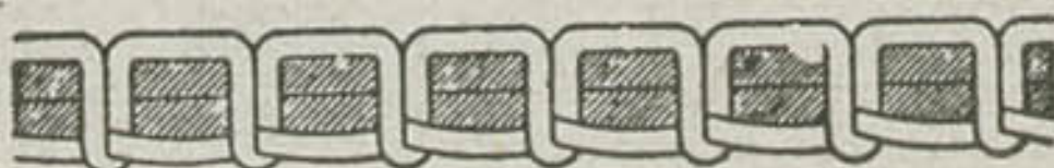
FIG. 13. LOOSE NEEDLE THREAD TENSION
