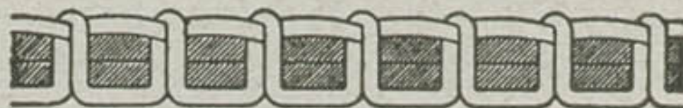
FIG. 12. TIGHT NEEDLE THREAD TENSION
