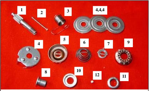
2 should be inside of 1. 4 #4s between sections of spring #3, and insert together, aligning tail of spring 3 in notches of stud 1 so that downward pressure is applied on thread by spring. Install 5, 6, 7, & 8. Get tension properly adjusted. Install dial 9 with about the indicator #4 up when adjusted for good straight stitch. Clamp with thumb nut 10. Insert #11, and secure with screw 12.
